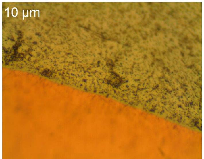
Properly Soldered at 450°F/232°C With Flux
